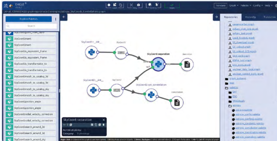
Figure 7: EAGLE, the graphical workflow editor for the DALiUGe system, developed by the ICRAR team. The very simple example graph shown computes the spherical distance of two coordinates on the sky and also identifies in which constellation one of them is located. This is performed by components from one of the most used astronomical software packages, astropy [13]
